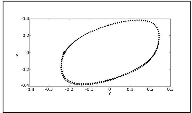
**Figure 3.** Poincaré section of sprung mass for  $\tau_u > \tau_s, \phi = 0.02$  (Period one).
