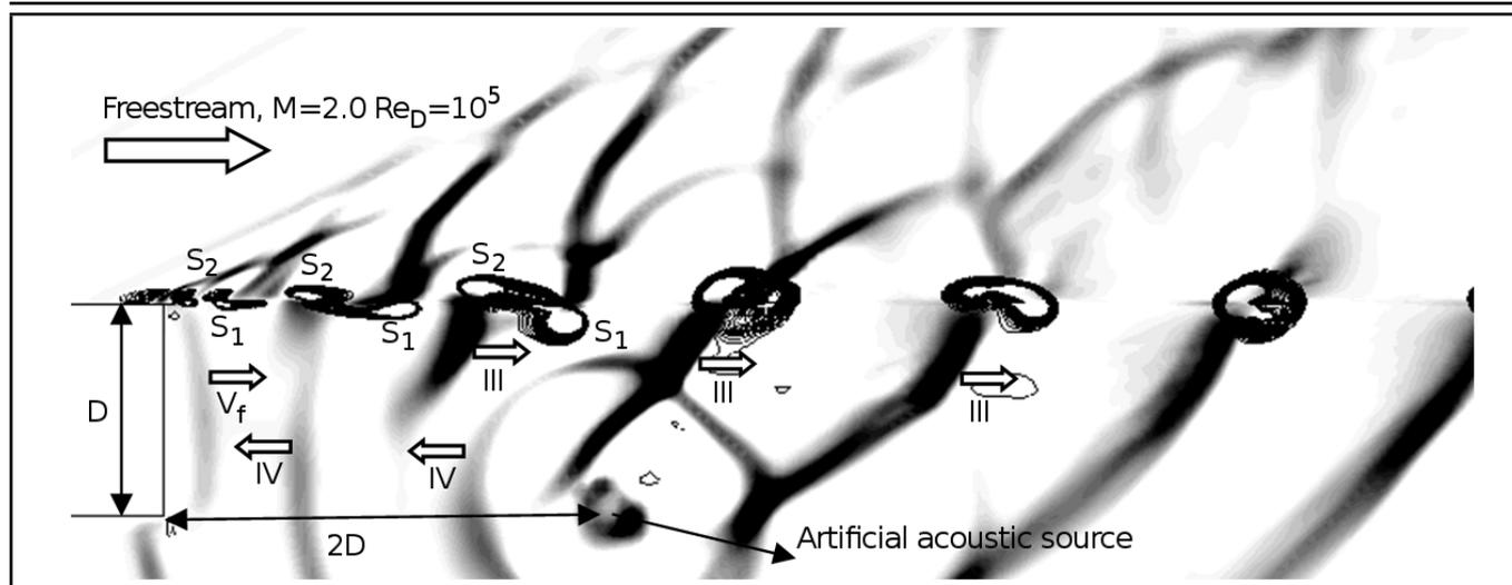
**Figure A1.** Free shear-layer subjected to an artificial acoustic source. Background contours represent the divergence of velocity ( $-2 < \text{div} \mathbf{u} < -0.1$ ), and black contour lines represent the second-order invariant of velocity gradient tensors ( $(a_\infty/D)^2 < Q_{2nd} < 15(a_\infty/D)^2$ ).
