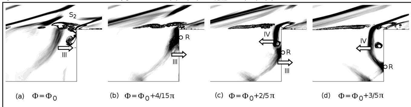
**Figure 12.** Reflection of Mach waves in the Ma3.0 case. Background contours represent the divergence of velocity ( $-2 < \text{div} \mathbf{u} < -0.1$ ), and black contour lines represent the second-order invariant of velocity gradient tensors ( $2(a_\infty/D)^2 < Q_{2nd} < 20(a_\infty/D)^2$ ).
