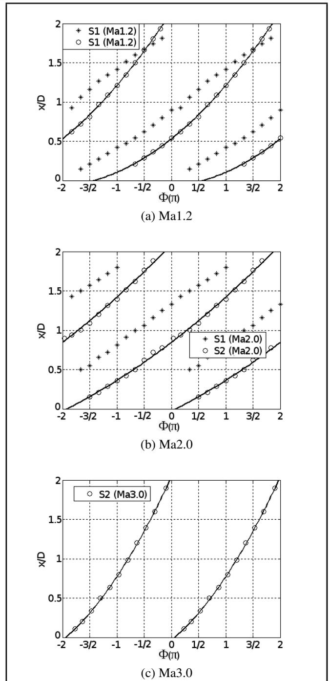
Figure 9. Convection trajectories of vortices in streamwise direction.
