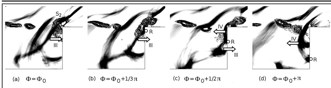
**Figure 11.** Reflection of Mach waves in Ma2.0 case. Background contours represent the divergence of velocity ( $-2 < \text{div} \mathbf{u} < -0.1$ ), and black contour lines represent the second-order invariant of velocity gradient tensors ( $2(a_\infty/D)^2 < Q_{2nd} < 20(a_\infty/D)^2$ ).
