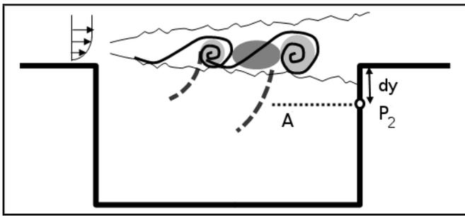
Figure 8. Schematic of large-scale vortices and Mach waves.
