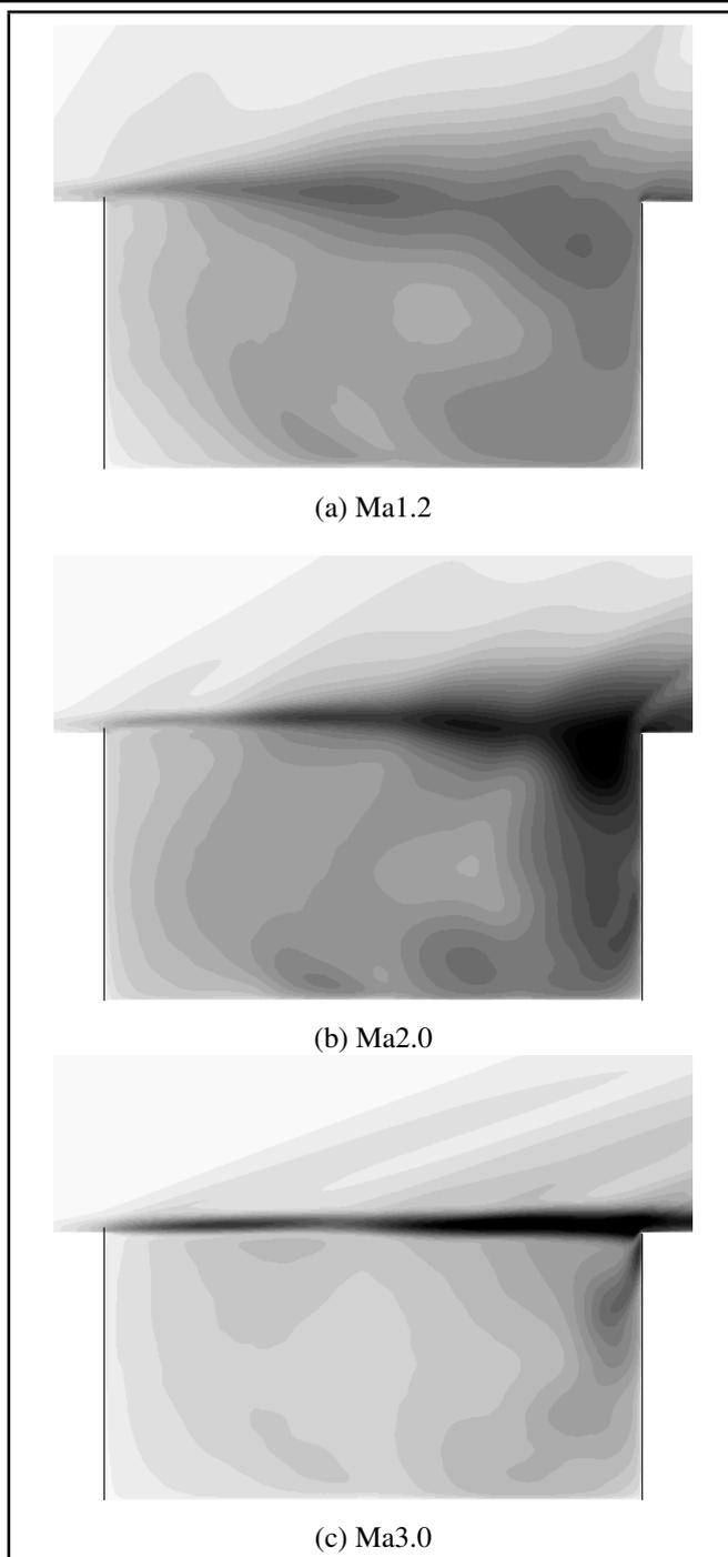
Figure 7. Contours of turbulence kinetic energy ( $0 < TKE < 0.5 a_\infty^2$ ).
