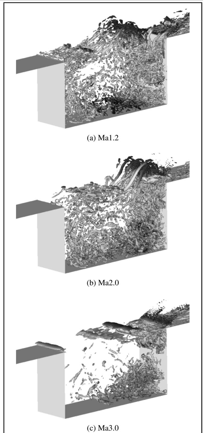
Figure 5. Snapshots of instantaneous flow-fields. Iso-surface of the second invariant of velocity gradient tensors,  $Q_{2nd} = 50(a_\infty/D)^2$ ; colored with streamwise velocity,  $-0.5 < u/u_\infty < 1$ .
