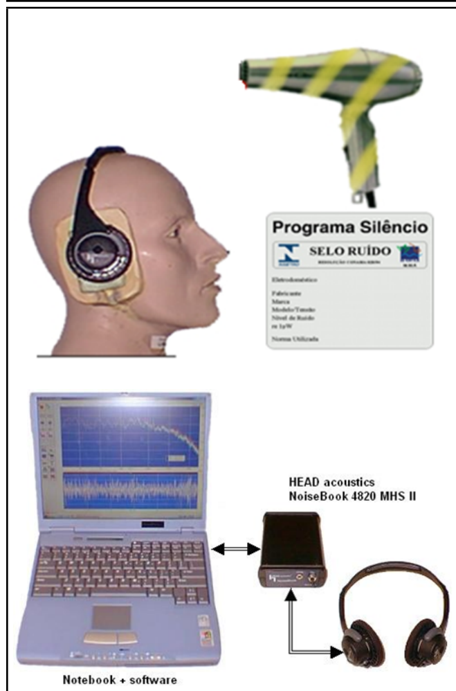
Figure 7. The binary recording of the sound using NoiseBook.
