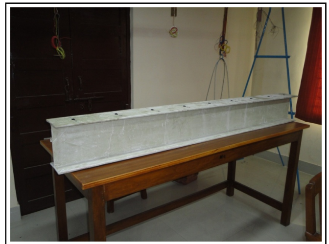
Figure 2. Fabricated FRP beam.
