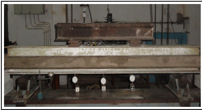
Figure 9. Experimental set up for four point bending test.
