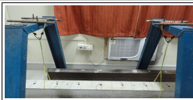
Figure 3. FRP beam suspended with rubber bands to simulate free-free boundary.
