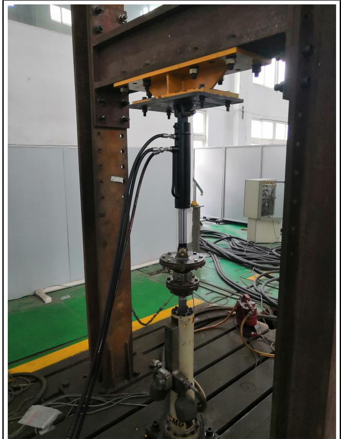
Figure 2. Electro-hydraulic servo equipment.
