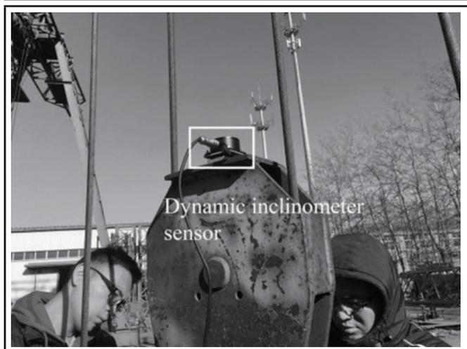
Figure 14. Installation of payload swing experiment subsystem.
